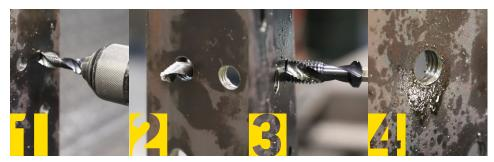
No pre-drilling necessary. The unique patented step tip design eliminates pre-drilling, so you can go straight into drilling. Next, it creates a perfectly centred, burr-free hole using a cordless drill and cutting fluid. The bit then smoothly threads and taps the hole—no jamming, no binding, and easy drill reversal from the threaded hole. Create a clean and smooth finish with the countersink feature ensuring a precise, flush chamfer.
