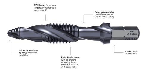
Drill, tap and countersink your way through mild steel, aluminium and stainless steel with the following features:
